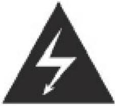
The lightning flash with arrowhead symbol within an equilateral triangle is intended to alert the user to the presence of uninsulated, “dangerous voltage” within the product's enclosure that may be of sufficient magnitude to constitute a risk of electric shock to a person.
