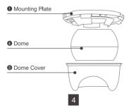
Step 4: Install the **1** Mounting Plate to the ceiling or wall in the position with the supplied screws.
