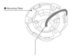
**Note:** The cable should be though the Mounting Plate.
