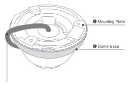
Note: The cable should be fixed on the slot hole.
