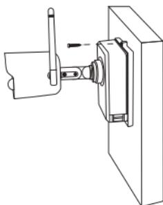
**3.2.4** Insert and tighten the screw on the bottom of the camera battery pack.
