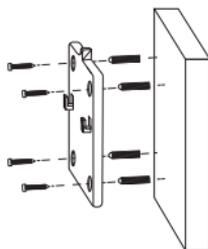
**3.2.2** Lock the two slots on the camera base to the hook on mounting base.
