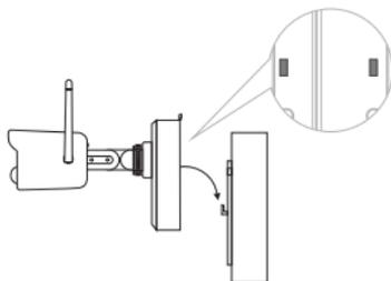
**3.2.3** Install and tighten the safety set screw.
