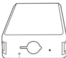
Screw hole on the bottom of battery pack
